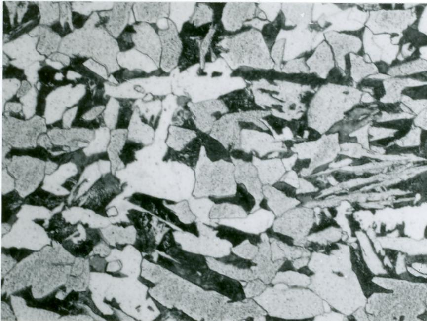
Figure 4.15 Microstructure of As-welded A515 Weld Joint
