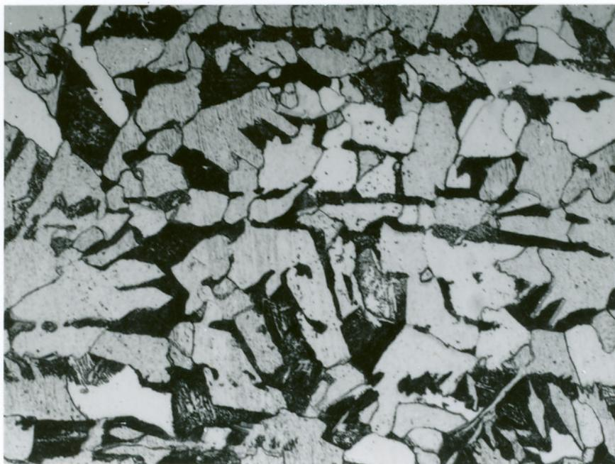
Figure 4.16 Microstructure of Stress-relieved A515 Weld Joint
