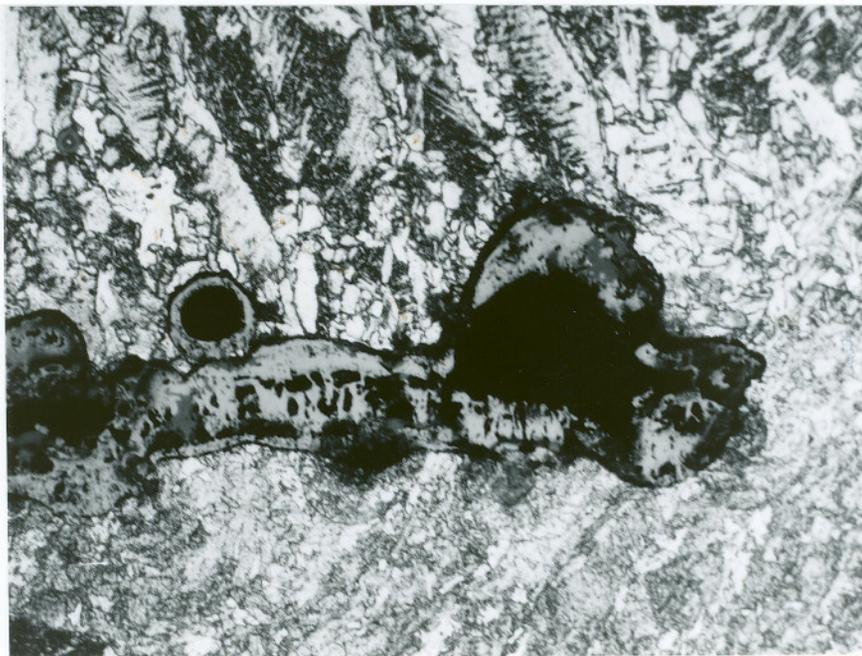
Figure 4.17 Weld Defect ( slag inclusion )
