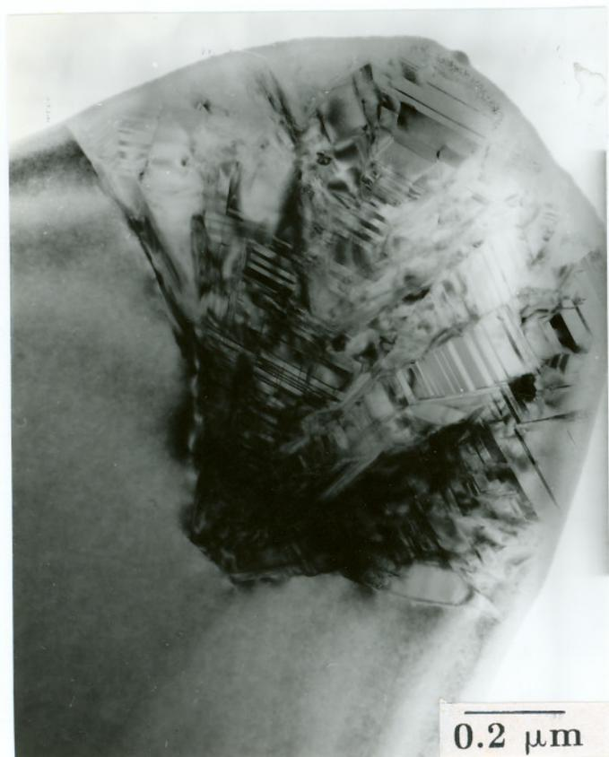
Figure 42. Cross-sectional TEM micrograph of a cone. The top portion is polycrystalline and the bottom is single crystal.
