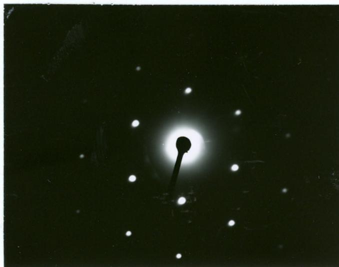
Figure 18. Transmission electron diffraction of the laser deposited GaP. The zone axis is [100].
