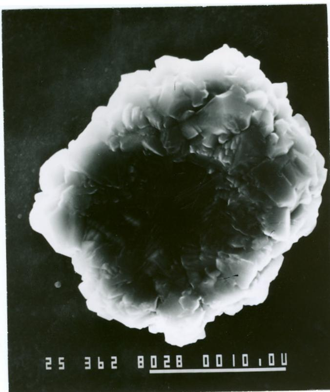
Figure 10. SEM micrograph of polycrystalline GaP grown using a stationary argon ion laser beam.
