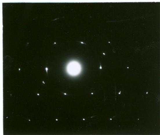
Figure 25. TEM diffraction pattern of a GaP microstructure on Si showing epitaxial alignment. The zone axis is [110].
