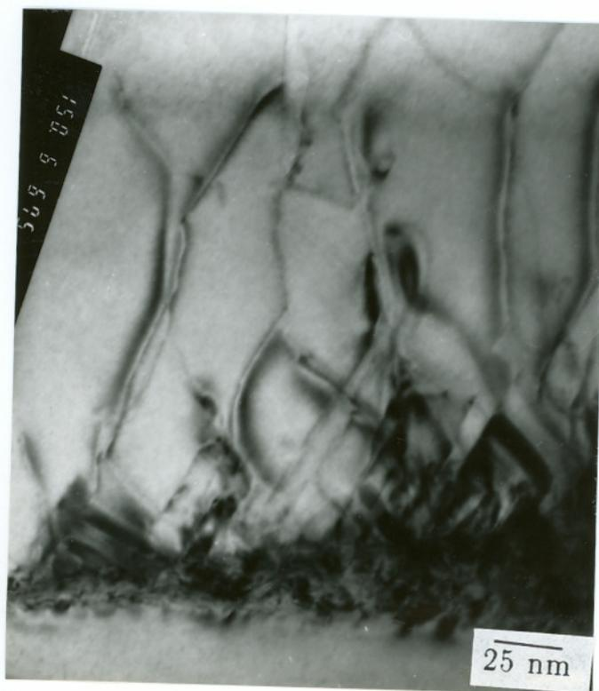
Figure 49. Cross-sectional TEM micrograph of GaP/GaAs tilted to reveal the interface.
