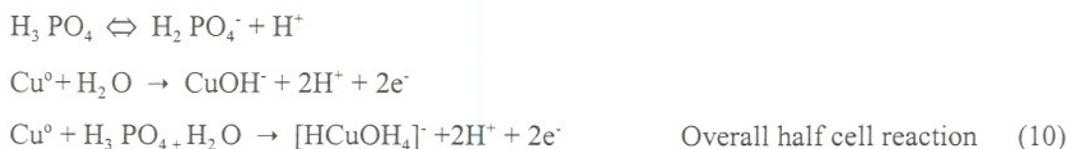
Reaction type 2 is similar to type 1 reaction for electropolishing of copper in phosphoric acid, however, the type 2 reaction does not include any reaction with water. The partial and overall reactions are shown below<sup>21,22</sup>:
