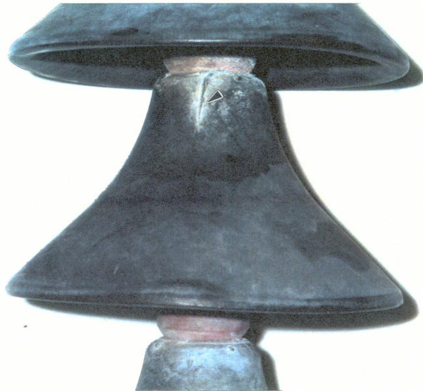
Figure 2.7 Surface cutting on the weathershed.
