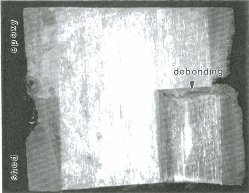
(b) Epoxy/sheath interface debonding
