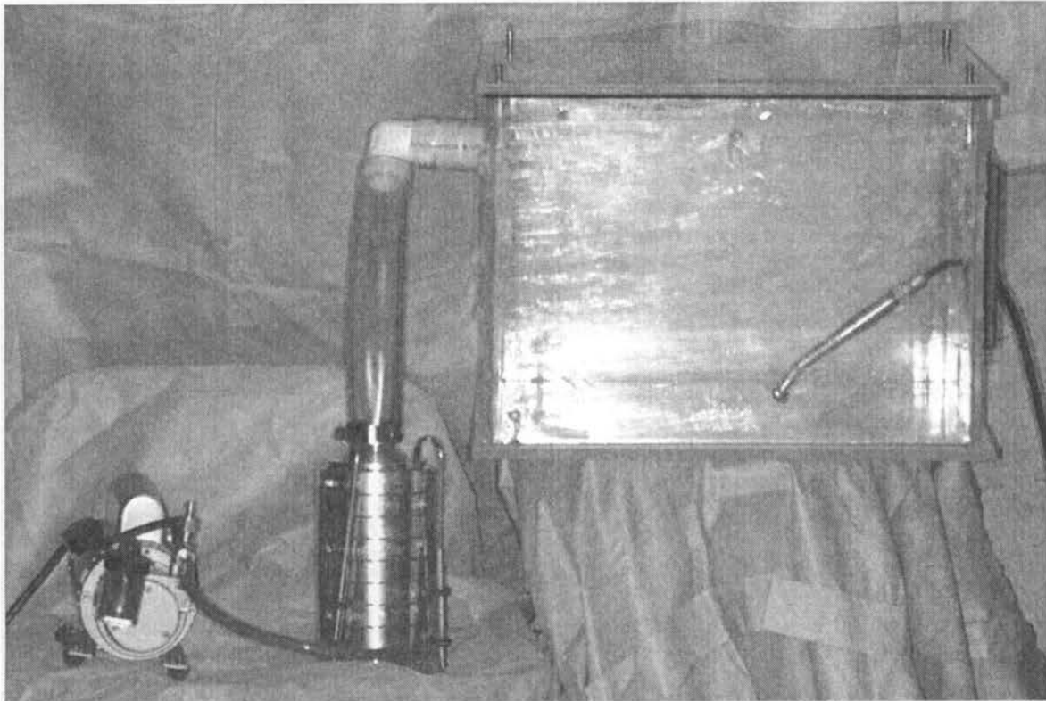
Figure 2. Test chamber with handpiece (R) with cascade impactor (center) attached to vacuum pump (L)
