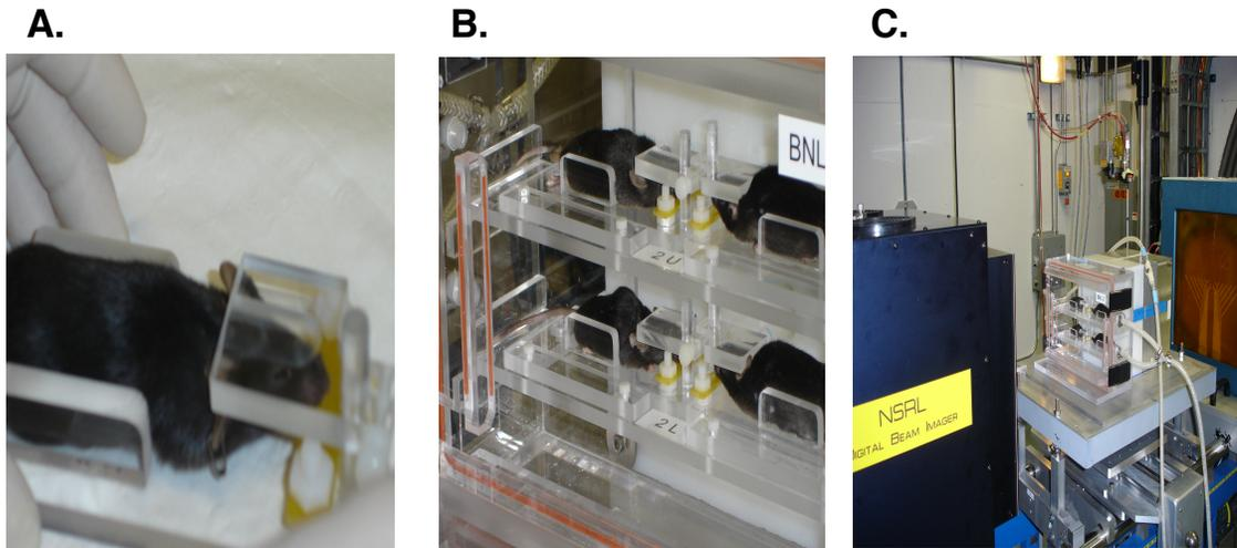
**Figure 20.** Set up of  $^{56}\text{Fe}$  irradiation of mice at Brookhaven National Laboratories. Mice were sedated and placed in positional cradles (A), which were loaded onto holding chambers (B) that had calibrated positions for the beam. The position of the holding chamber was then placed in the beam line (C).
