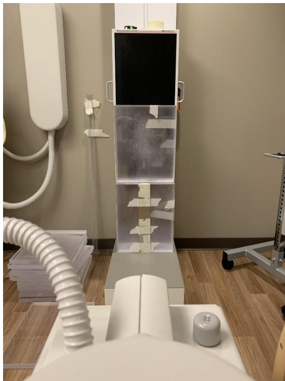
Figure 4 Here the configuration is displayed for 8/9 acrylic at 80 inches. Note that the aluminum strip is centrally placed.
