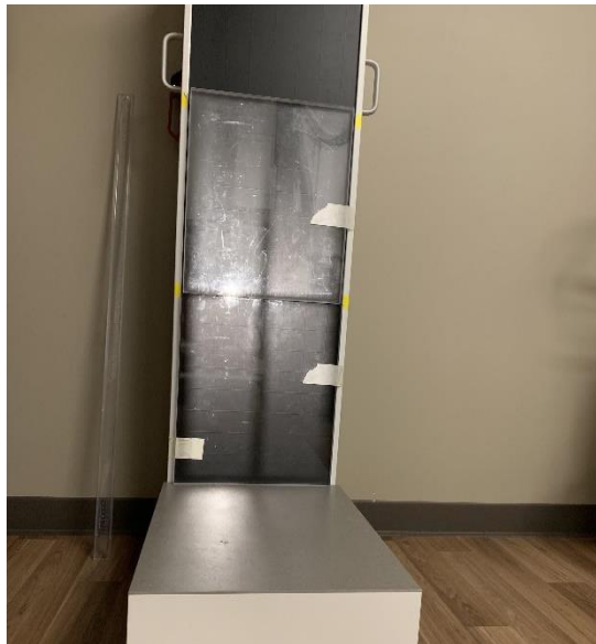
Figure 3 Note the width collimation on the bottom block where the penumbra of the light field is positioned within the acrylic. A slight bottom border is also visible. This was collimation adjusted for an SID of 72 inches.
