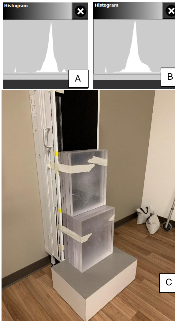
Figure 8 Both histogram displays share the same techniques. Source to Image distance of 72 inches, tube potential 85 kVp and 80 mAs. A) Histogram distribution for five acrylic blocks on top of nine (5/9). B) Histogram distribution for three blocks on top of eleven (3/11). C) Shows acrylic configuration for 5/9.
