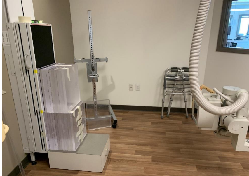
Figure 5 Overview of the experimental set up portraying the techniques for ten blocks placed on top of eleven blocks, 10/11 acrylic configuration with an SID of 72 inches. It was later apparent that more acrylic was necessary to prevent excess scatter from the top row. The 4.445 mm of 1100 alloy aluminum was also added in order to compensate for extra attenuation due to the vertebrae.
