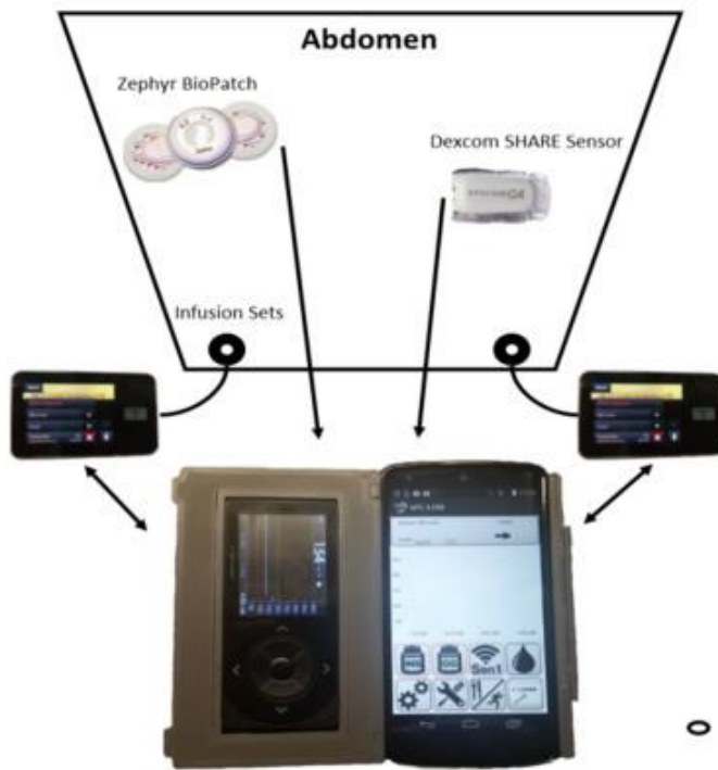
Figure 1.1 Hardware components of the OHSU dual-hormone AP
