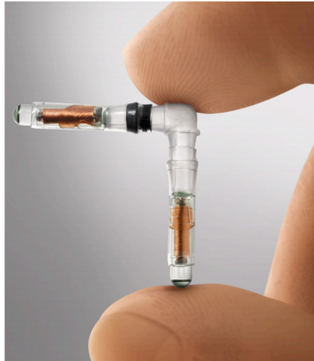
Figure 2.5: Calypso surface beacon transponder. Image accessed May 2017, available at https://www.varian.com/sites/default/files/resourceattachments/CalypsoSurfaceBeaconTransponderRAD10289Mar2013.pdf .
