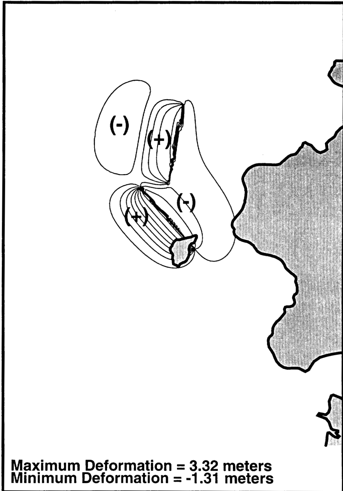
FIGURE 3.6 Bottom Deformation for DCRC-2 Source
