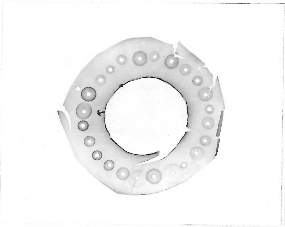
Radial immunodiffusion gel after staining and drying showing distinct variation in the size of precipitin rings.
