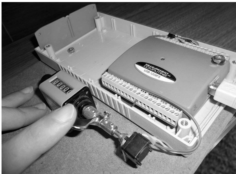
Figure 3.1. A close up of the instrumented replica of the Halstead-Reitan manual finger tapper. The cover has been removed to show the internal electronics.
