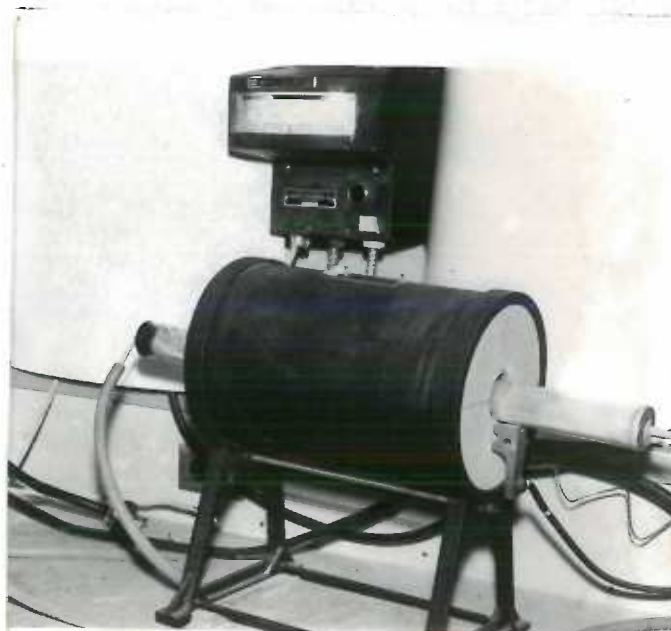
Fig. 4 Horizontal oven used to heat amalgam specimens
