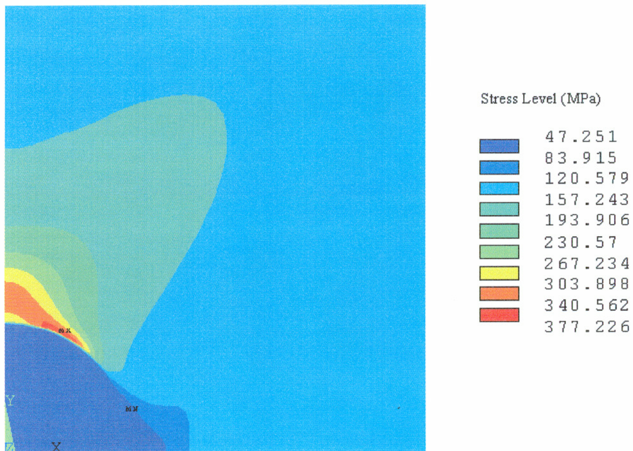
Figure 5-10 Hydrostatic stress contour around a graphite particle (Applied stress = 450 MPa).
