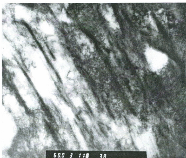
Figure 3-15 Dissolving cementite in Steel 1 after deep cold deformation but before spheroidizing annealing.
