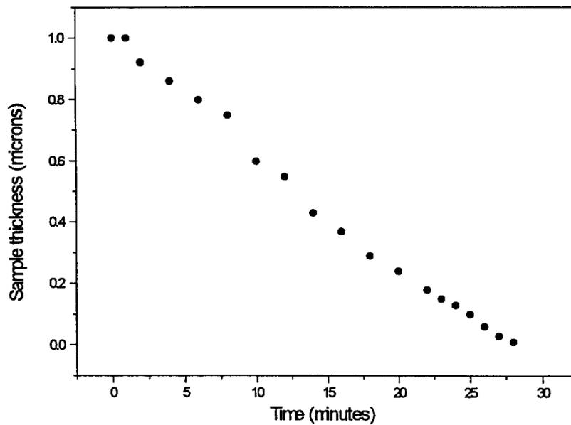
Figure 2.6 Thickness of Ag Film vs. Time
