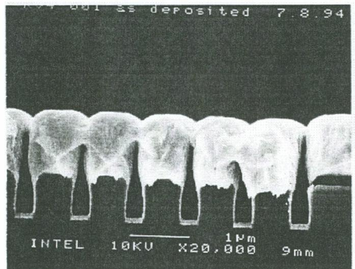
Figure 4.2 Sample KV4-001 as deposited (Ti/Ag/TiN//oxide)
