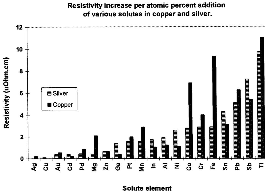
Figure 5.1 Resistivity increase per atomic percent addition of various solutes in copper and silver
