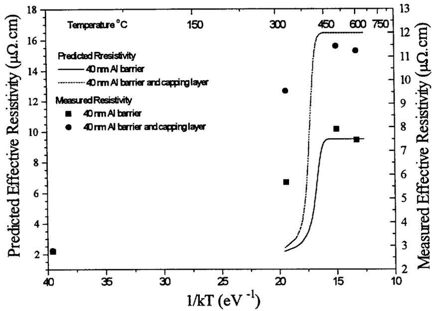
Figure 5.11 Graph of predicted and measured effective resistivity vs.  $1/kT$
