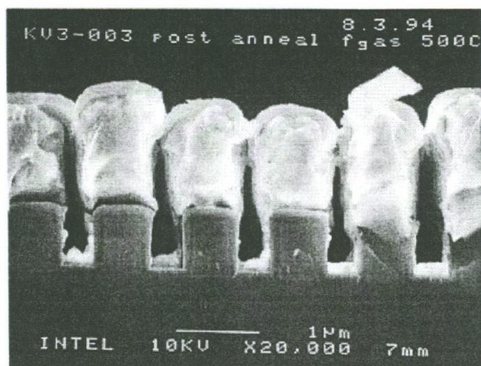
Figure 4.7 Sample KV3-008 annealed (TiW/Ag/Ti//TiN//oxide)
