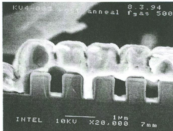
Figure 4.9 Sample KV4-003 annealed (Ti/Ag/TiN)
