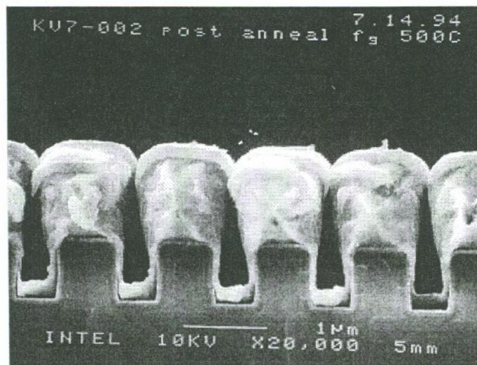
Figure 4.15 Sample KV7-002 annealed (TiW/Ag/TiW//oxide)
