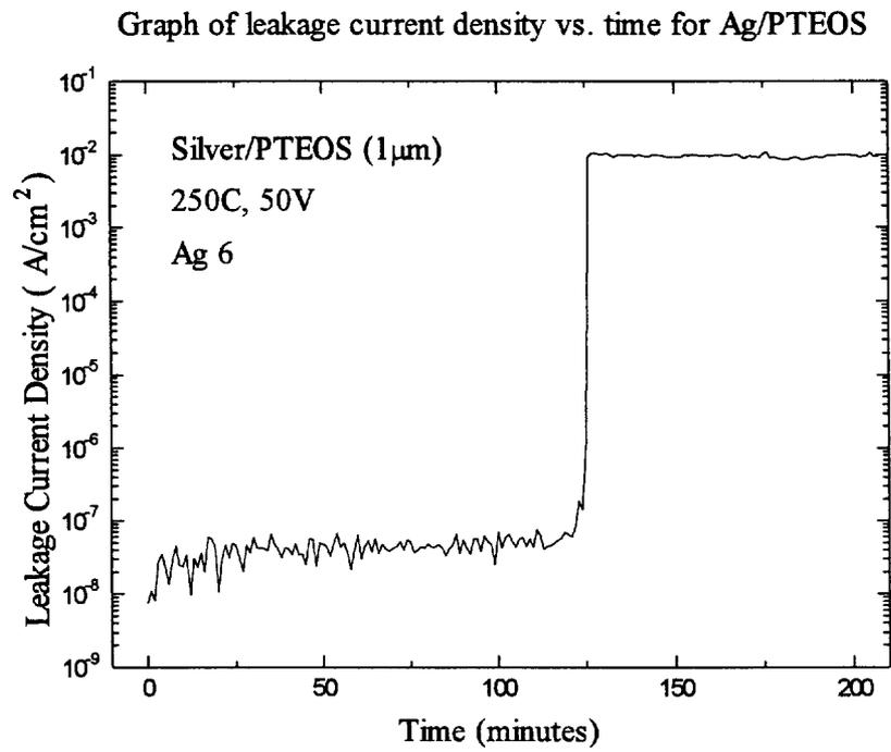
Figure 3.2 Leakage current density vs. time curve for BTS of 250 °C, 0.5 MV/cm (evaporated Ag/1  $\mu$ m PTEOS oxide/Si)
