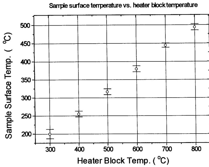
Figure 2.3 Sample Surface vs. Heater-Block Calibration.
