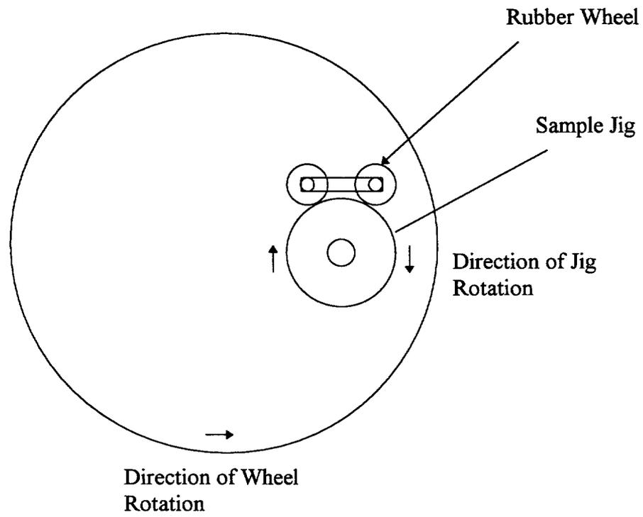
Figure 2.5 Polishing Wheel Set-Up
