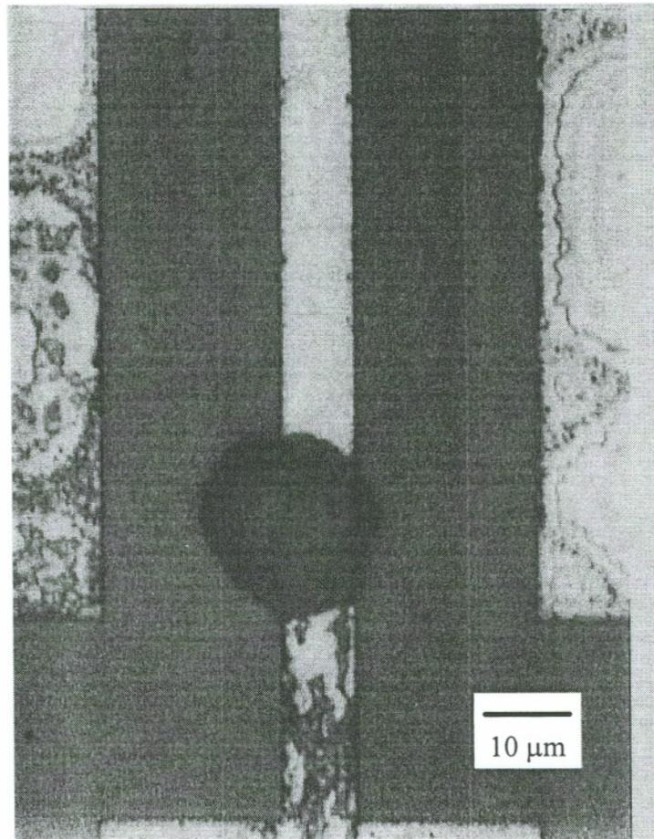
Figure 3.26 Ag protrusion on EM structure
