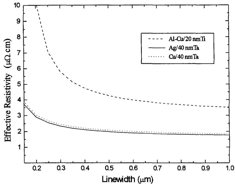
Figure 1.3 Graph of effective line resistivity at room temperature vs. linewidth for Al-Cu with 200 Å Ti wetting layer, Cu with 40 nm Ta diffusion barrier, and Ag with 40 nm Ta diffusion barrier
