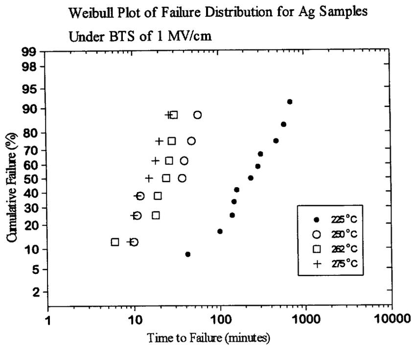
Figure 3.22 Weibull plot of cumulative failure vs. time for Ag-based MOS structures.
