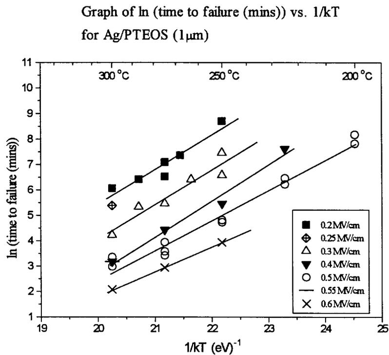
Figure 3.7 Graph of natural log of time to failure vs.  $1/kT$
