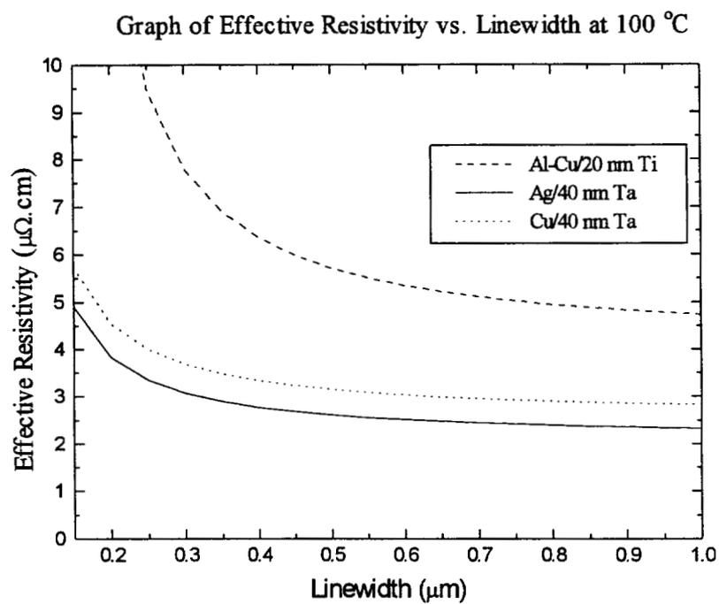
Figure 1.4 Graph of effective line resistivity at 100 °C vs. linewidth for Al-Cu with 200 Å Ti wetting layer, Cu with 40 nm Ta diffusion barrier, and Ag with 40 nm Ta diffusion barrier
