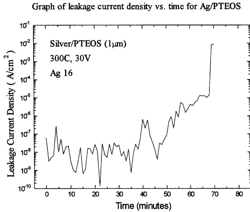
Figure 3.4 Leakage current density vs. time curve for BTS of 300 °C, 0.3 MV/cm (evaporated Ag/1  $\mu$ m PTEOS oxide/Si)
