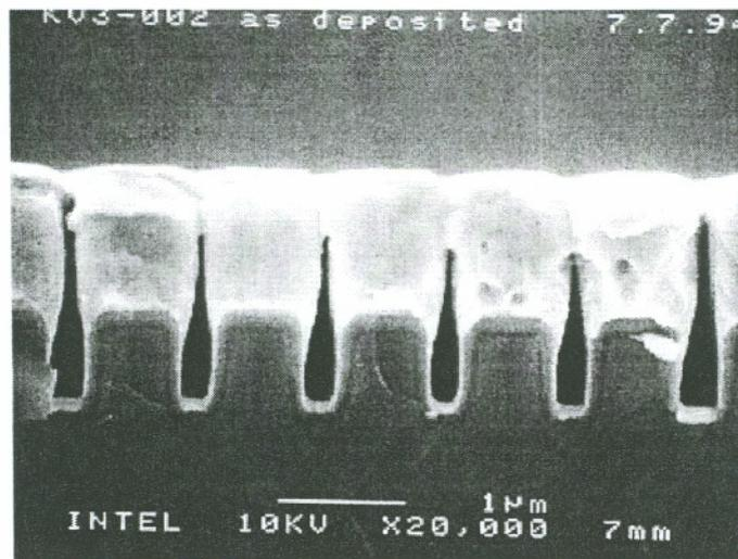
Figure 4.1 Sample KV3-002 as deposited (TiW/Ag/Ti//TiN//oxide)
