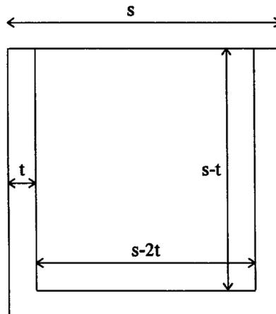
Figure A1.1 Conducting line with barrier thickness,  $t$
