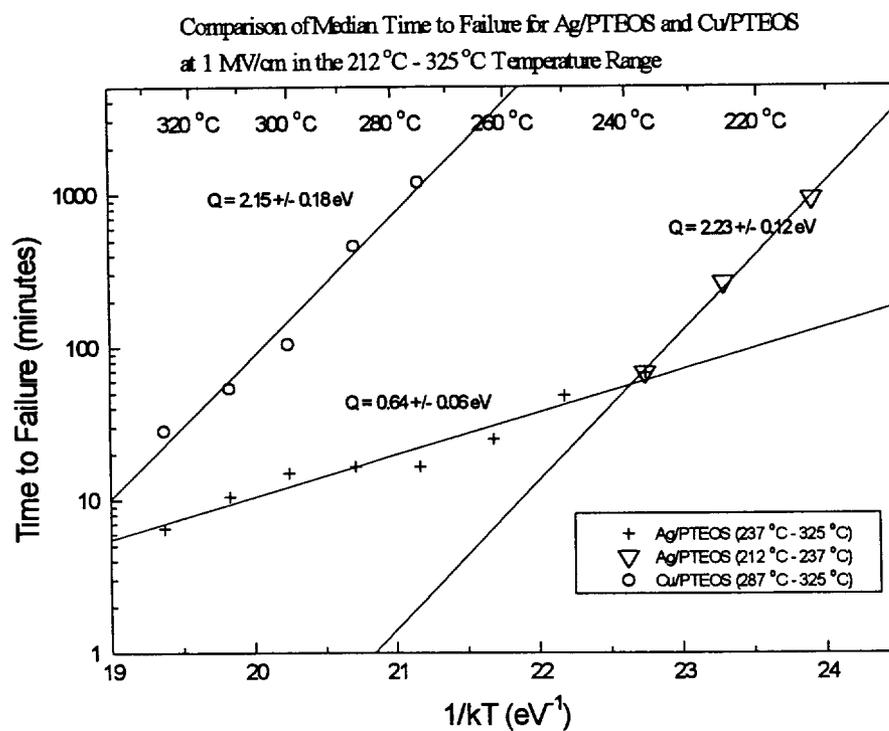
Figure 3.20 Median time to failure vs.  $1/kT$  for Ag/PTEOS and Cu/PTEOS
