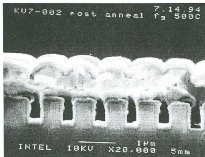
Figure 4.14 Sample KV7-002 annealed (TiW/Ag/TiW//oxide)
