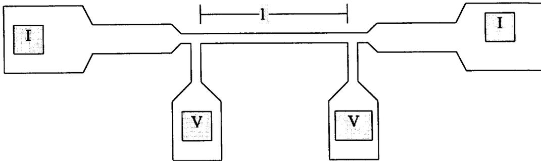
Figure 3.23 Electromigration (EM) test structure
