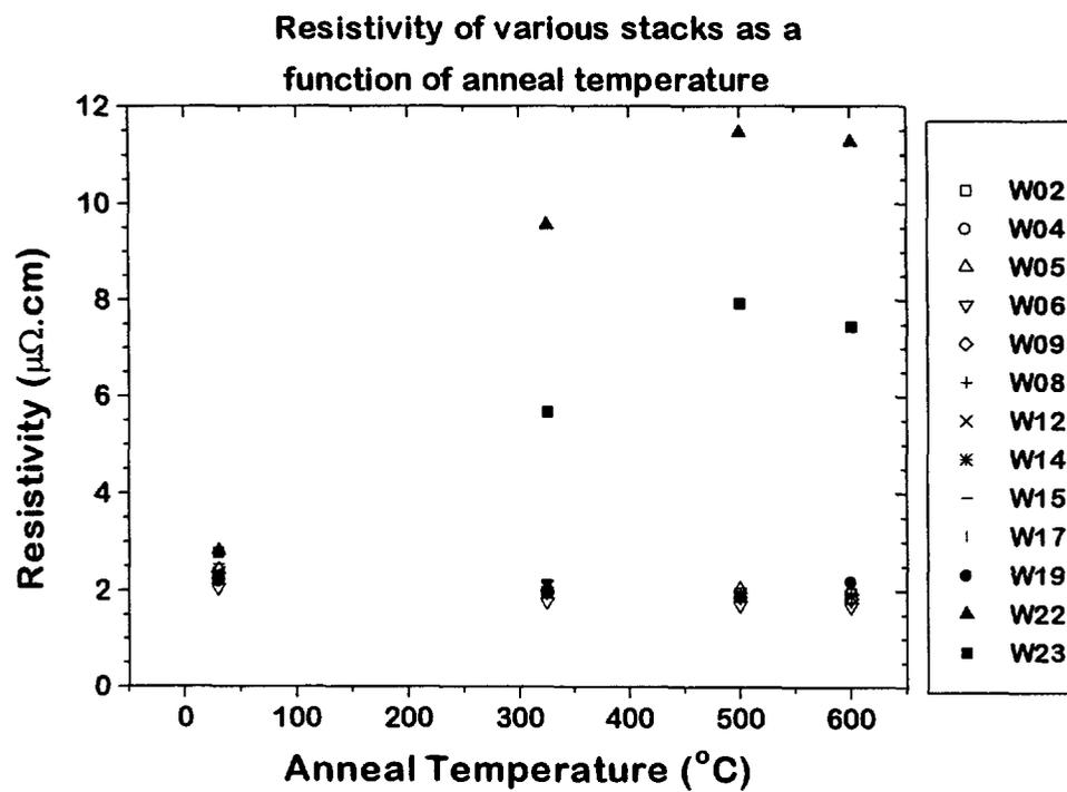
Figure 5.4 Resistivity of various stacks after 2 hour forming gas anneal (recipes of wafer numbers are given in Chapter 2, Table 2.1)
