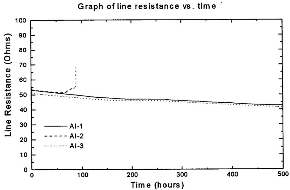
Figure 3.25 a) Ag line resistance data, 200 °C, 20mA/ $\mu\text{m}^2$
