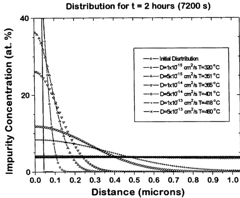
Figure 5.7 Solution to the diffusion equation for a 40 nm barrier layer for a 2 hour anneal.
