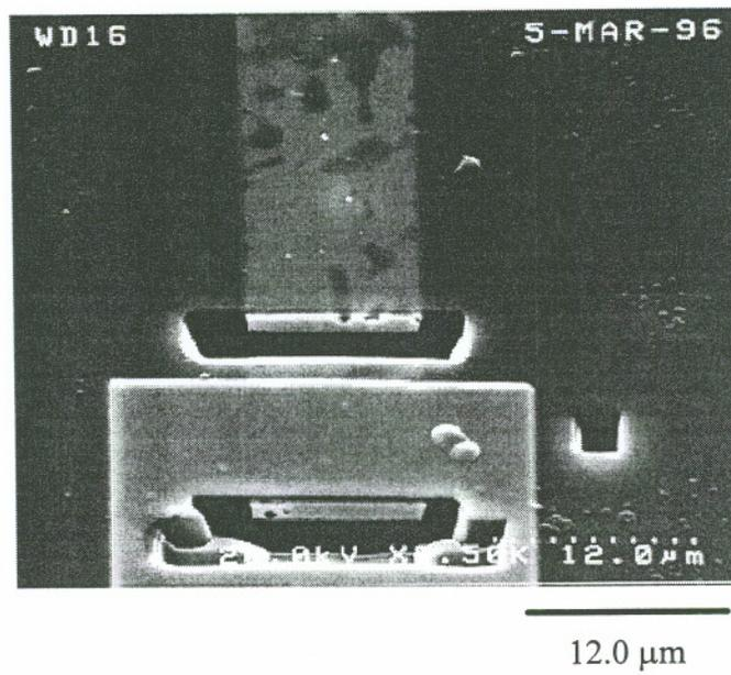
Figure 3.29 Cross-section of EM structure
