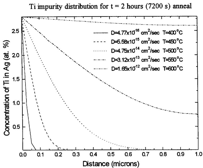
Figure 5.13 Ti impurity distribution for a 2 hour anneal
