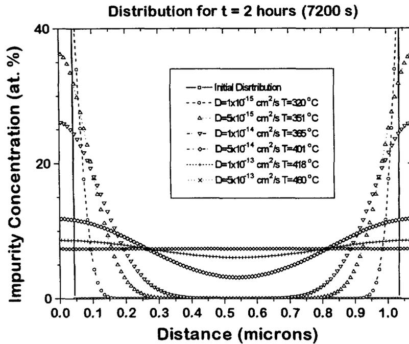
Figure 5.9 Solution to the diffusion equation for a 40 nm barrier layer and 40 nm capping layer for a 2 hour anneal
