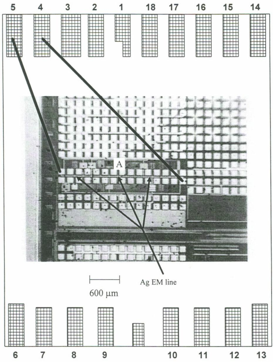
Figure 3.24 Micrograph of the EM test structure
