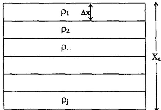
Figure 5.10 Cross-section of a conducting film
