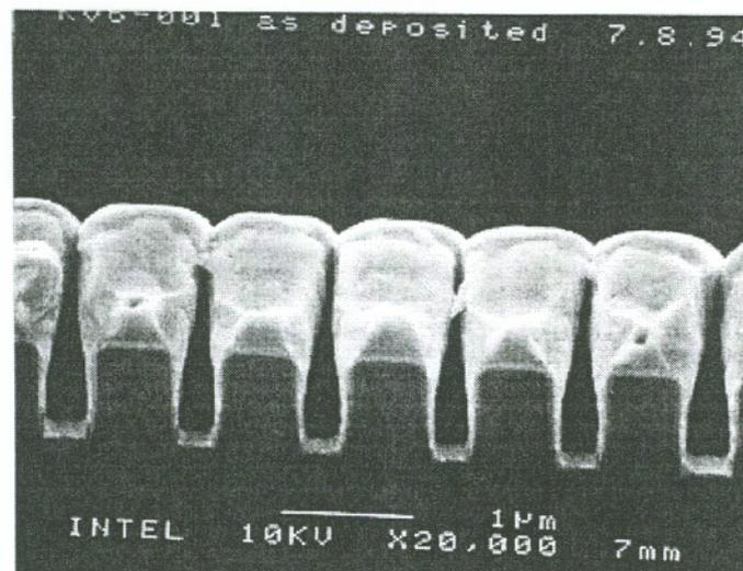
Figure 4.4 Sample KV6 as deposited (TiW/Ag/TiW//oxide)
