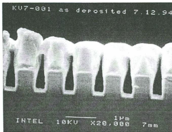
Figure 4.5 Sample KV7-001 as deposited (TiW/Ag/TiW//oxide)
