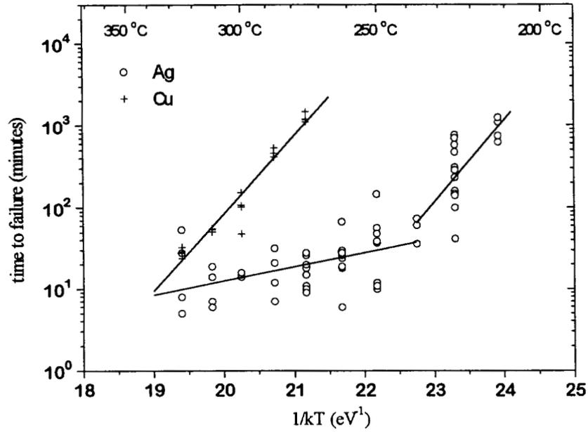
Figure 3.12 Graph of time to failure vs.  $1/kT$  for Ag and Cu (1 MV/cm, 0.5 micron PTEOS)
