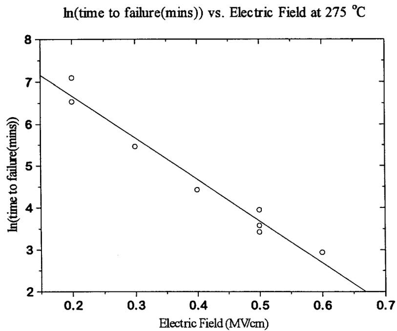
Figure 3.10 ln(time to failure(mins)) vs. electric field at 275 °C
