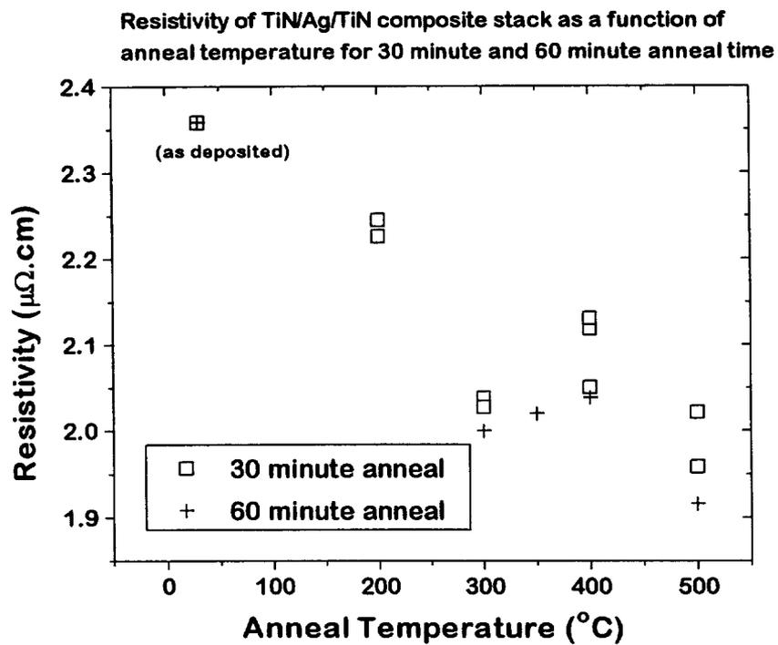
Figure 5.2 Resistivity of TiN/Ag/TiN (W12) samples for UHV anneal
