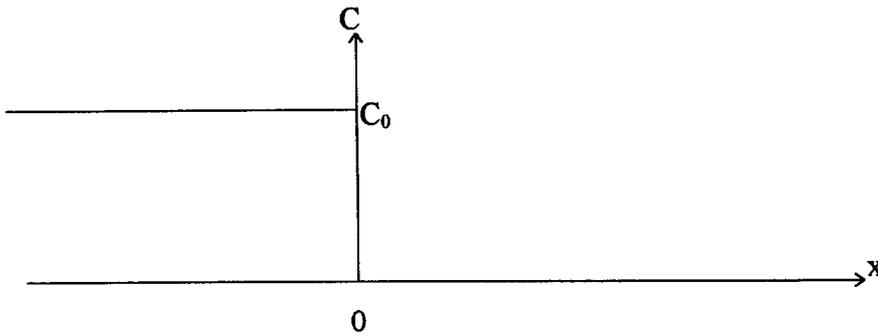
Figure A2.2 Initial conditions of an Interface.
