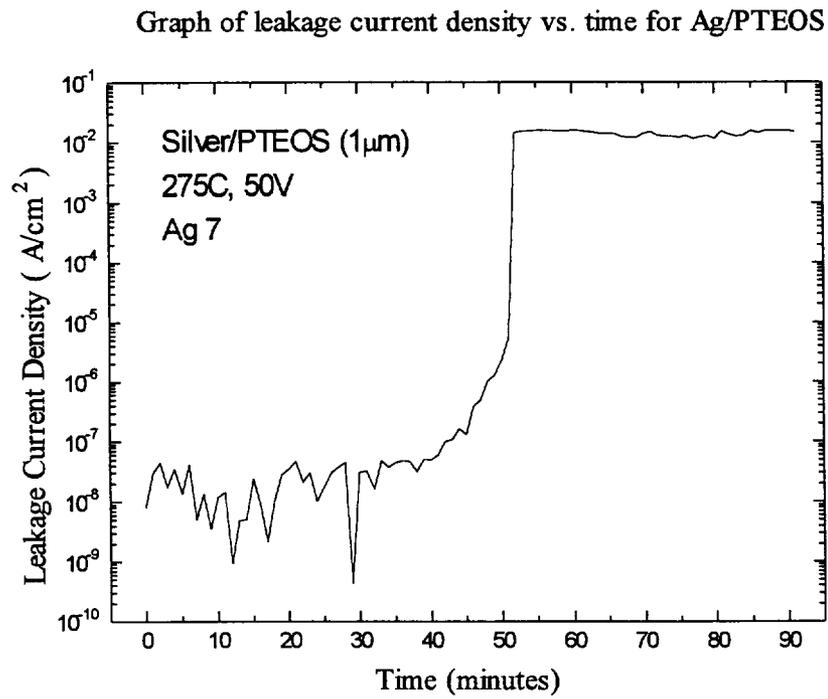
Figure 3.3 Leakage current density vs. time curve for BTS of 275 °C, 0.5 MV/cm (evaporated Ag/1  $\mu m$  PTEOS oxide/Si)
