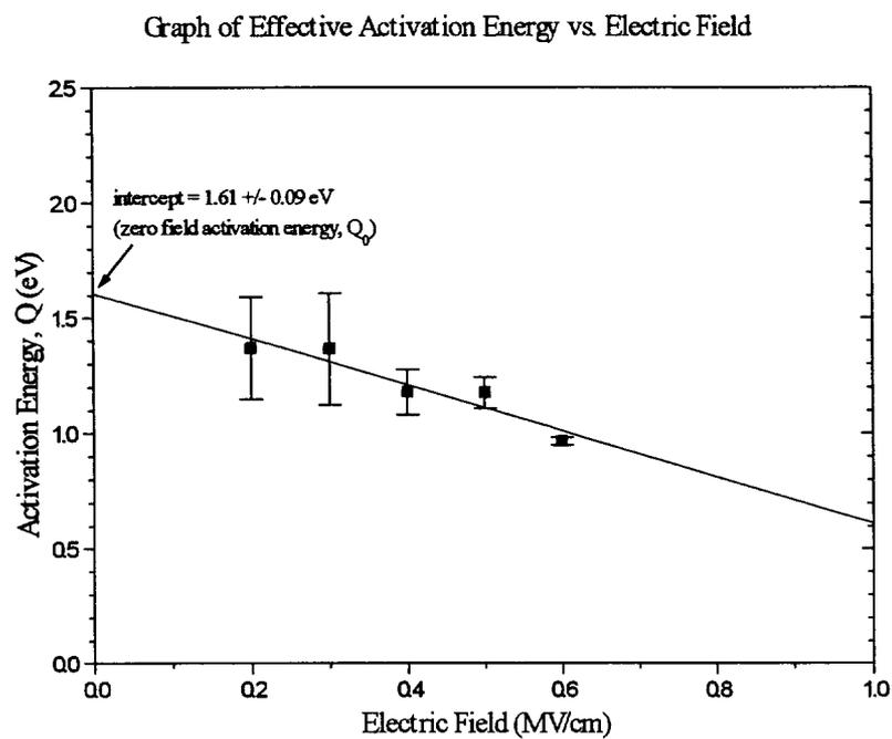
Figure 3.8 Graph of effective activation energy vs. electric field (evaporated Ag/1  $\mu$ m PTEOS oxide/Si)
