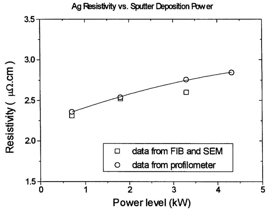
Figure 2.4 Graph of Resistivity of Ag Film vs. Sputter Deposition Power
