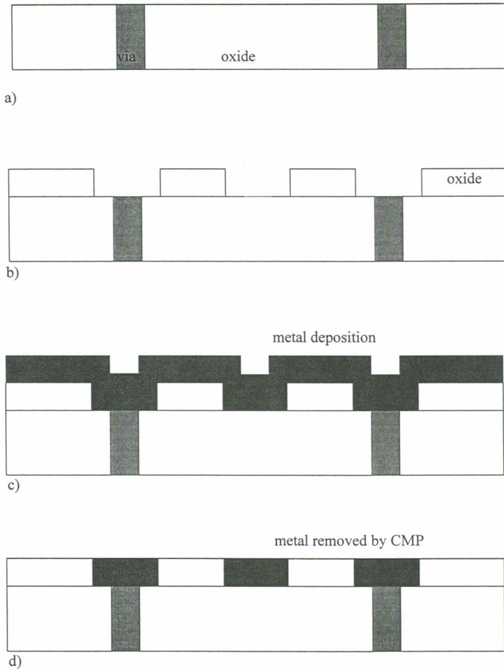
Figure 1.2 Steps for Al line realization. (a) vias are etched into oxide then filled with either W or Al, (b) oxide deposition and patterning, (c) Al deposition, (d) excess Al removed by CMP
