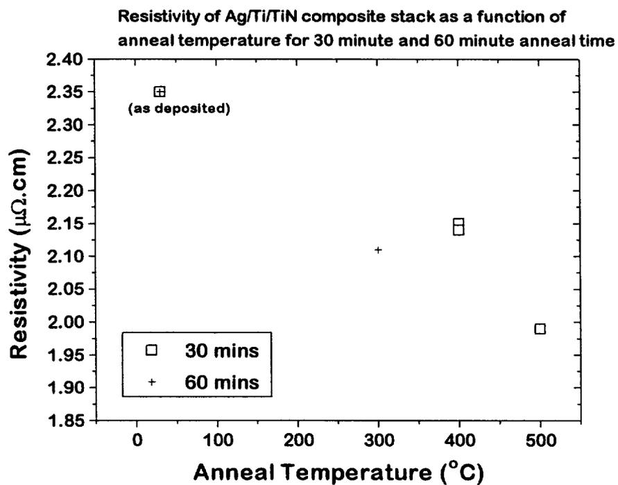
Figure 5.3 Resistivity of Ag/Ti/TiN (W19) stacks for UHV anneal
