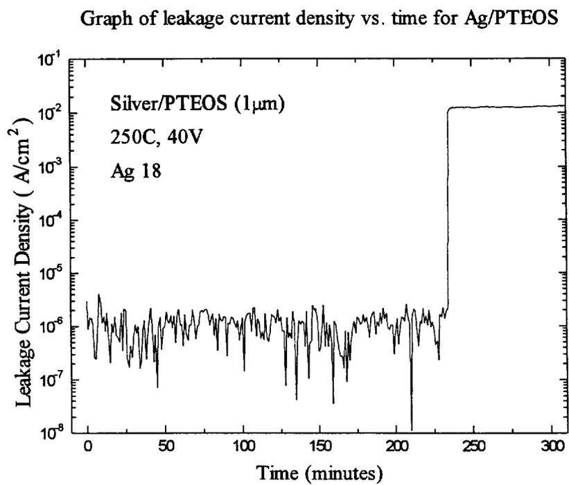
Figure 3.1 Leakage current density vs. time curve for BTS of 250 °C, 0.4 MV/cm (evaporated Ag/1  $\mu$ m PTEOS oxide/Si)
