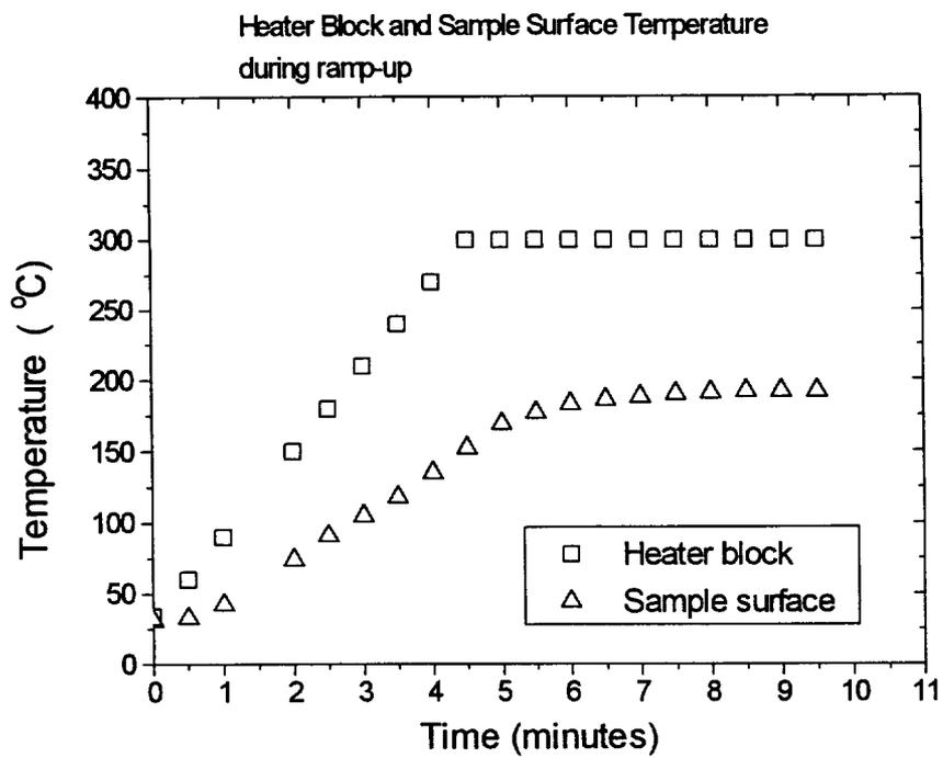
Figure 2.2 Temperature of Heater Block and Sample Surface During Ramp-Up
