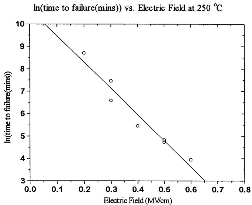
Figure 3.9 ln(time to failure(mins)) vs. electric field at 250 °C
