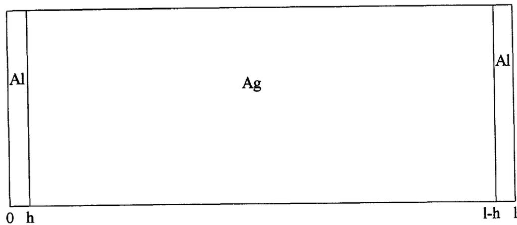
Figure 5.8 Schematic representation of Al/Ag/Al structure.
