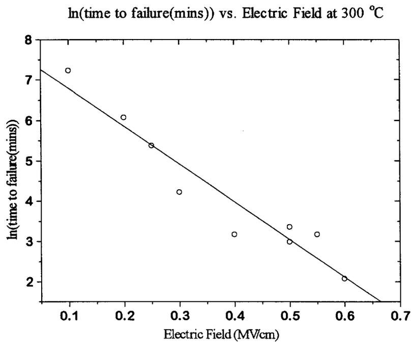
Figure 3.11 ln(time to failure(mins)) vs. electric field at 300 °C
