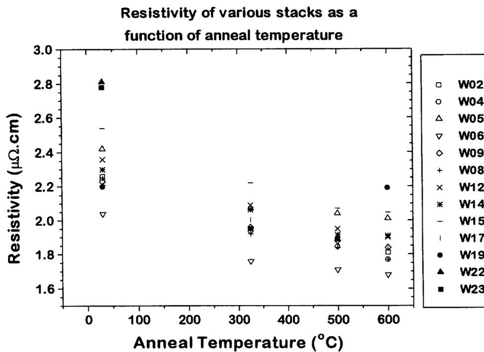
Figure 5.5 Resistivity of various stacks after 2 hour forming gas anneal.
