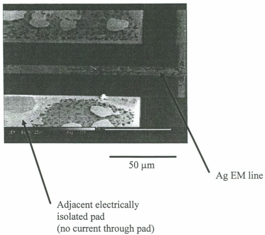
Figure 3.28 Ag EM structure and adjacent bondpads
