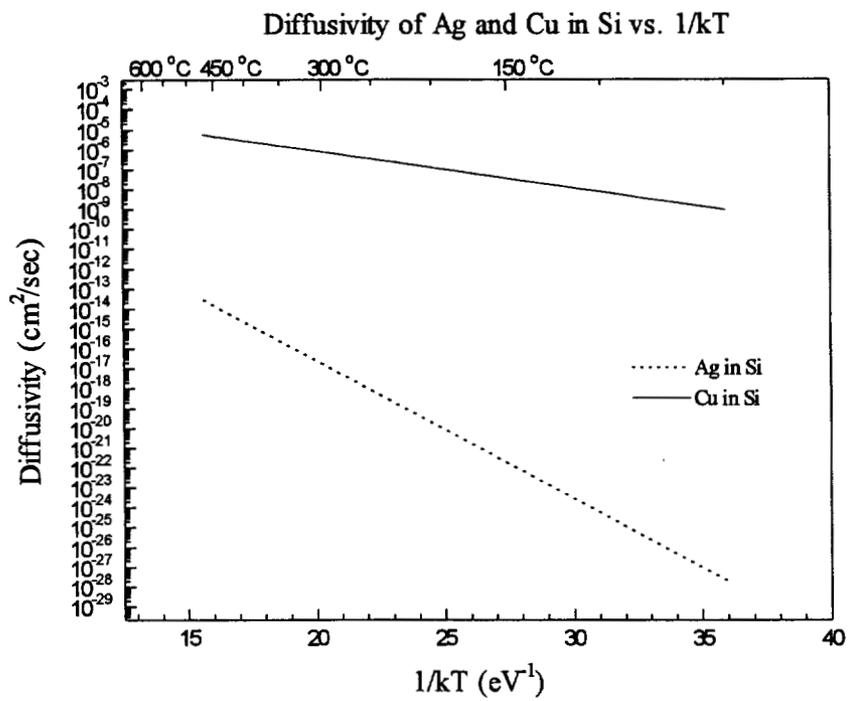
Figure 3.21 Diffusivity of Cu and Ag in Si
