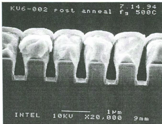
Figure 4.13 Sample KV6-002 annealed (TiW/Ag/TiW//oxide)
