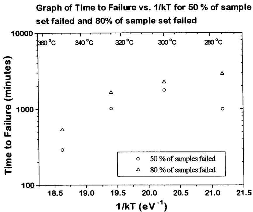
Figure 5.16 50 % time to failure and 80 % time to failure vs.  $1/kT$  for Ta barrier, 1 MV/cm
