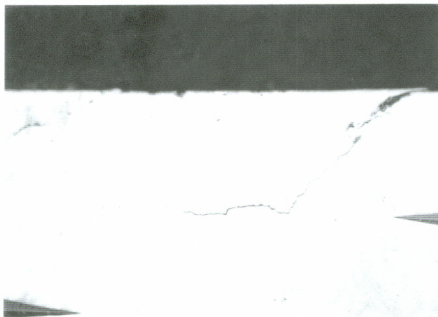
Figure 2.18 A subsurface crack appeared to have been initiated by a surface inclusion. Magnification 400x.
