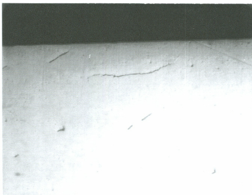
Figure 2.20 A subsurface crack in roller M1-9004C. Magnification 200x.
