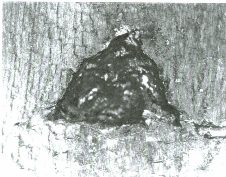
Figure 2.47a A typical type II spall of an arrow head appearance. Magnification 15x.
