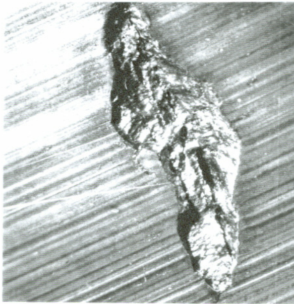
Figure 2.45a Another typical type I spall. Magnification 15x.
