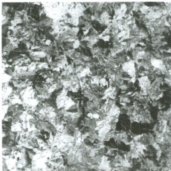
Figure 2.4a Microstructure of M3-C90 steel at a magnification of 100x.
