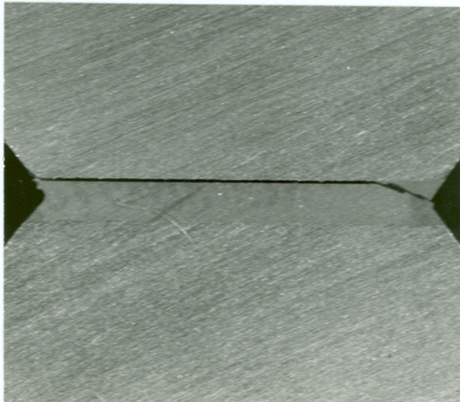
Fig. 3.59 Zig-zag crack path (rigid adhesive, t=1.0 mm, \phi=-30^\circ ).
