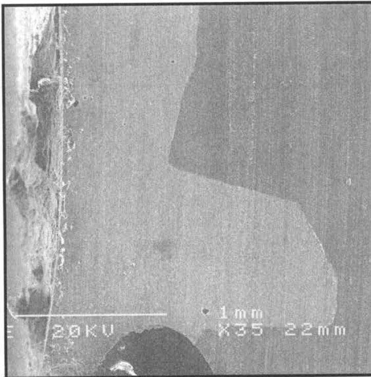
Figure 6. Homogenous mixture of particulate (80% strontium) with resin (X35).
