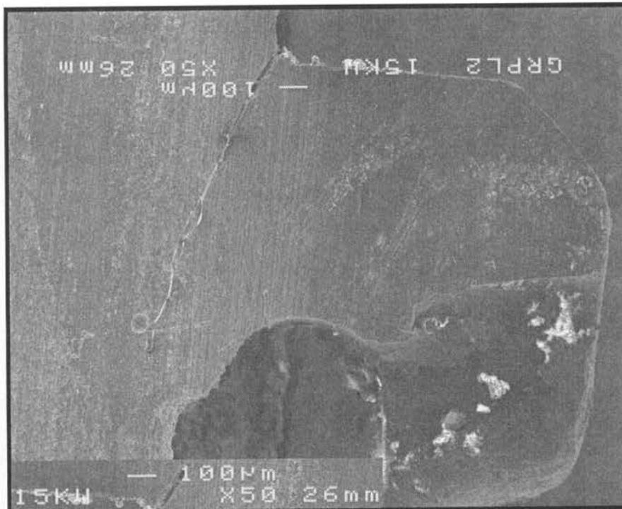
Figure 12. Random orientation of E-glass fibers. Di-methacrylate resin-rich areas present (X50).
