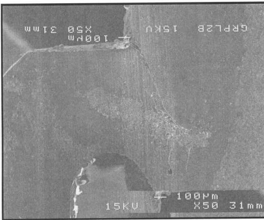
Figure 11. Poor placement of E-glass fibers within tie-wing complex; fibers located far from initial site of fracture (X50).
