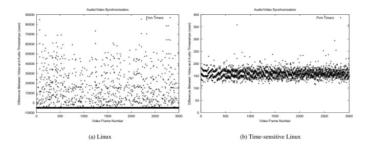
Figure 3: Audio/Video Skew on Linux and time-sensitive Linux. Background load copies a 8 MB buffer from user level to a file with a single write call. Note that the two figures have different scales, and that the maximum skew in Figure (b) is much smaller than in Figure (a)
