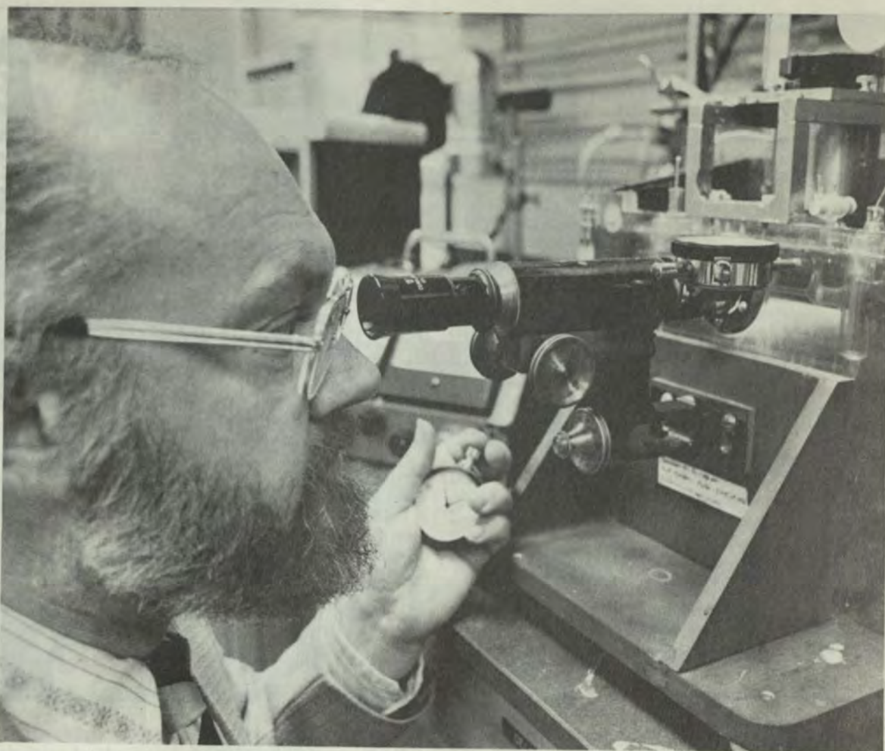
Dr. Geoffrey Seaman, advisor to NASA on space research, clocks red blood cells moving across an electrical field on an apparatus he designed which has modified for use in space by NASA.
