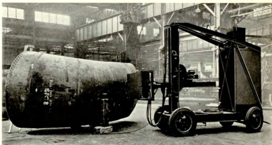
PLATE 27. Here is a mobile X-ray unit being used to X-ray a welded joint. It was machinery like this which was employed to examine the welds at Boulder Dam. It is machinery like this which is now X-raying boilers for the Navy and weldings for Victory ships and airplanes. (Photograph, courtesy of the General Electric Xray Corporation.)
