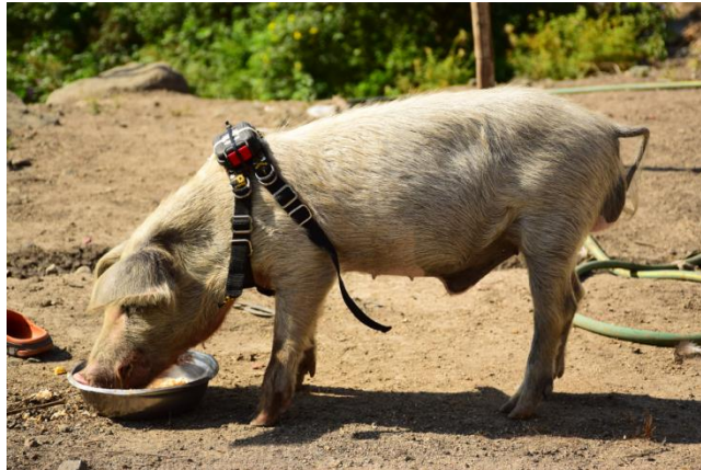
Fig 3.1. GPS devices placed in waterproof cases and secured to harnesses for tracking.
