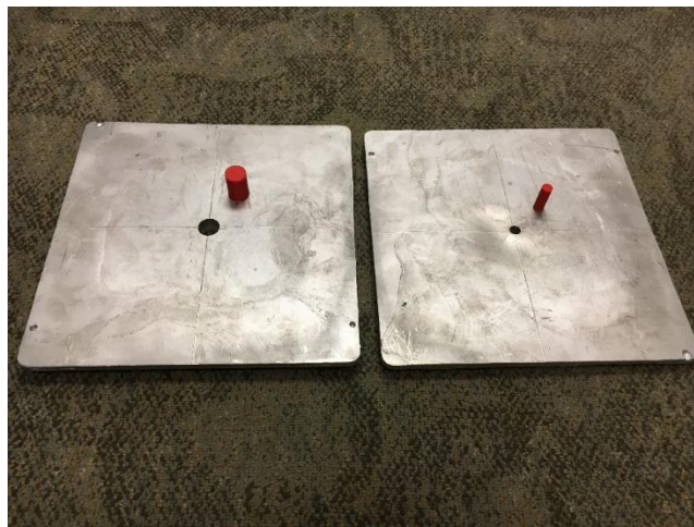
Figure 9. The cutouts created for the measurement of the LBR. The 3D printed cylinders were lined closely to the center.
