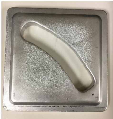
Figure 15. The irregular cutout. The corner measurement was taken in the bottom right corner, indicated by the black dot.
