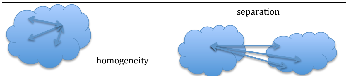
Figure 6. A) homogeneity is mean distance of observation to its own cluster center. B) separation is the average distance between the cluster centers, normalized for the number of cluster members. Silhouette width incorporates both the distance of observations to their own cluster center and to neighboring cluster centers.
