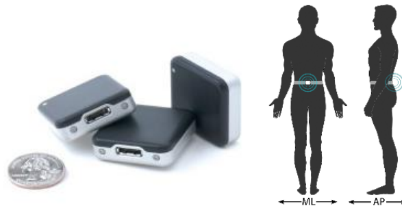
Figure 1.2: Inertial sensors are validated as an alternative postural sway measurement device to the “gold standard” force plate. A wireless, body-worn inertial sensor (Opal sensor, APDM, Inc.) mounted to the approximate location of the body’s CoM ( i.e. , the trunk, or more specifically, near the L5 lumbar spine) is used to quantify Acc-based postural sway measures.
