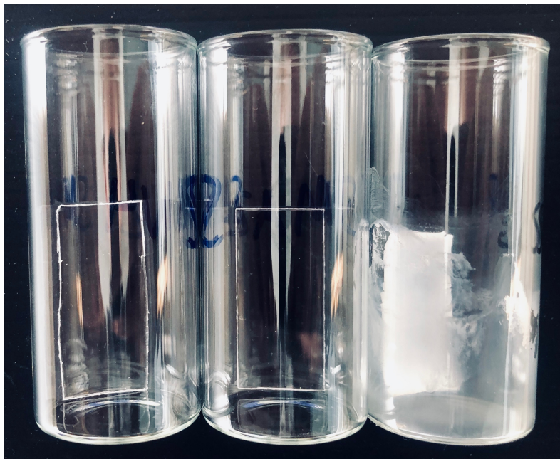
Figure 16. Depicts 14-day Smart Move samples that were in water, ethanol and dichloromethane, from left to right, respectively
