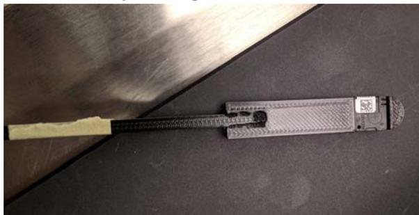
**Figure 24. nanoDot Orientation in Holder**
