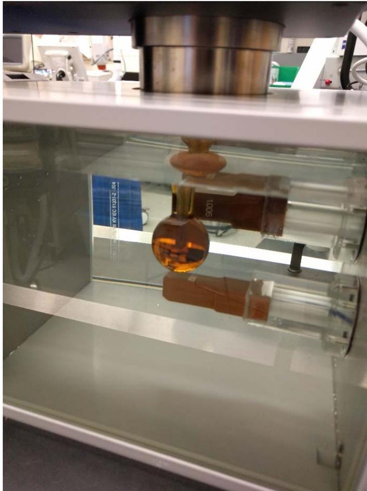
**Figure 9. Spherical Applicator in Water Tank**
