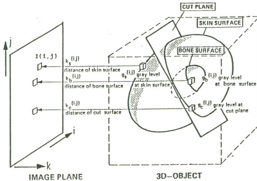
Figure 5.1 Geometry for tomographic surface reconstruction. [Hoehne et al. 1987]
