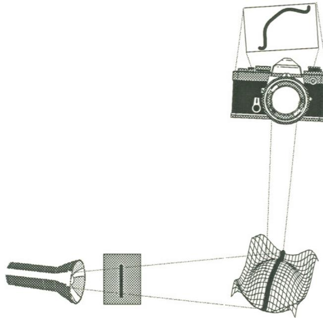
**Figure 8.1 Schematic of single line structured light apparatus**
