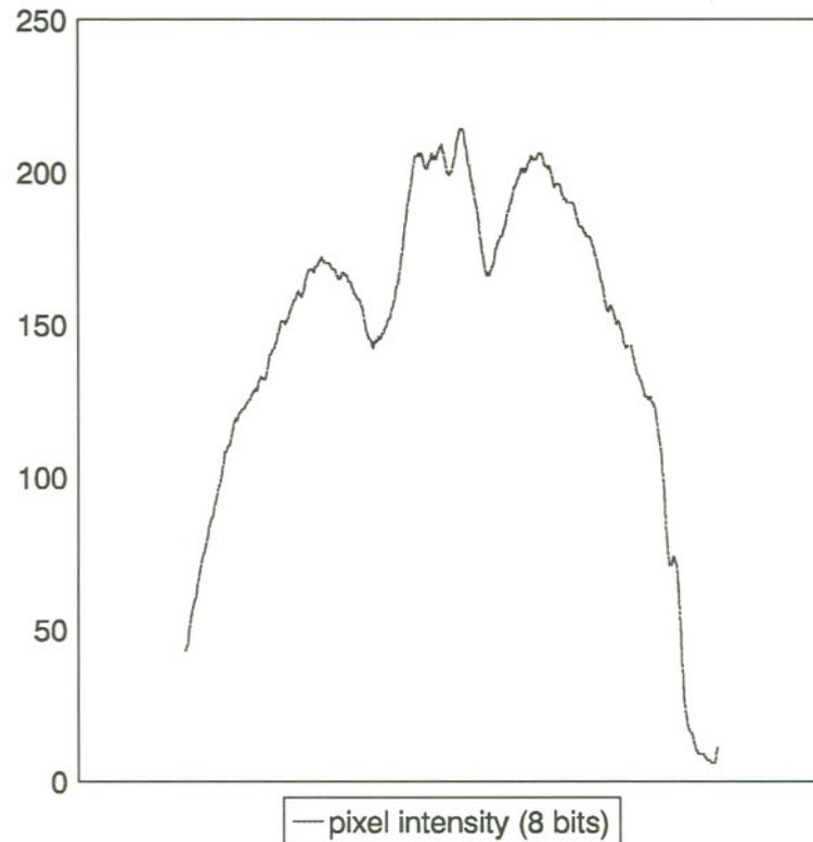
**Figure 7.4 c Scan line pixel intensities with 5 x 5 smoothing**
