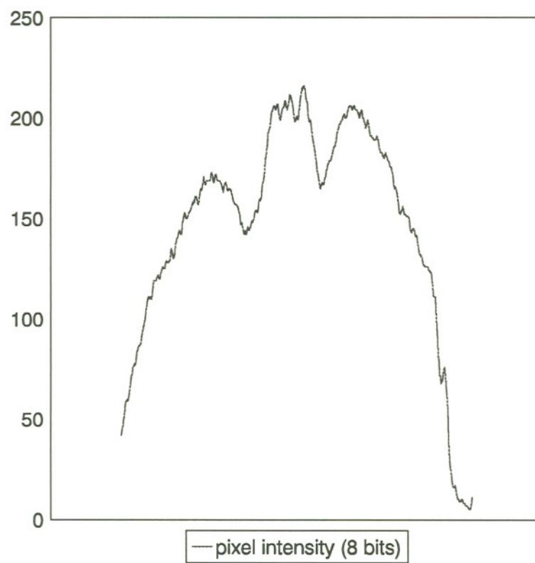
**Figure 7.4 b Scan line pixel intensities with 3 x 3 smoothing**
