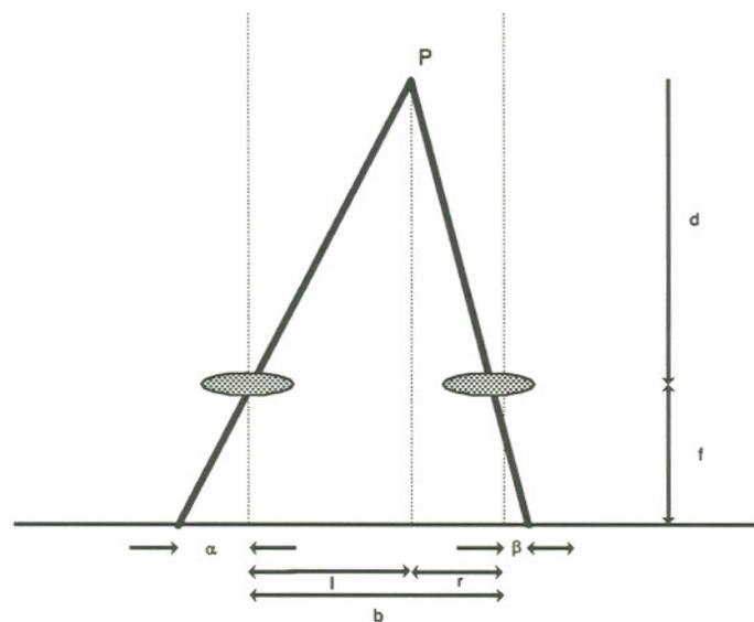
**Figure 7.2 The geometry of stereometric imaging**
