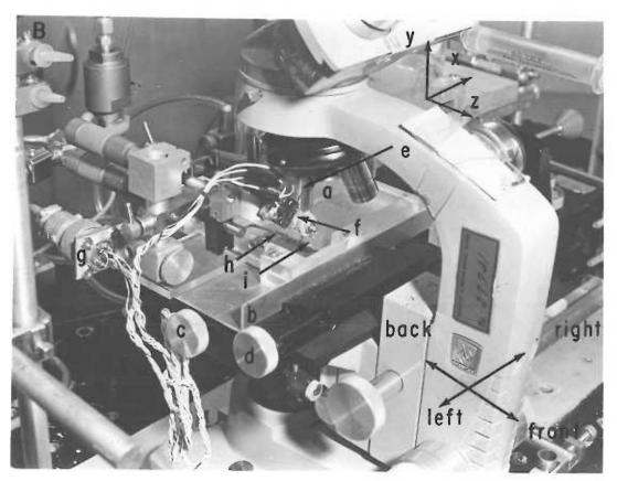
Figure 11. Fiber mounting apparatus in the experimental chamber. Minute rubber bands (a) clamp the terminal tufts (b) of an isolated fiber segment (c) to the stainless steel extension arms (d).
