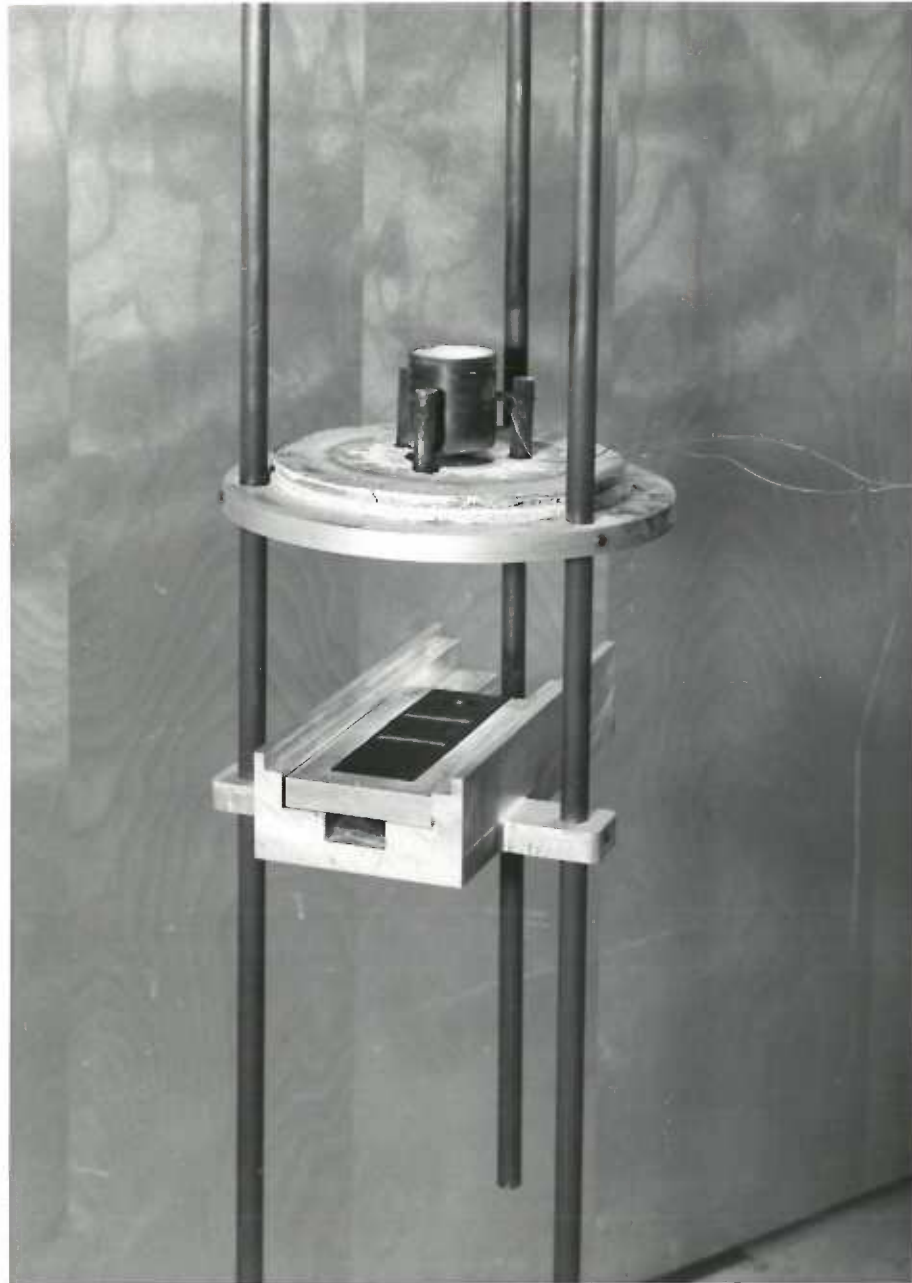
PLATE 3. Oven Platform, Mounted Ring, Cassette In Place
