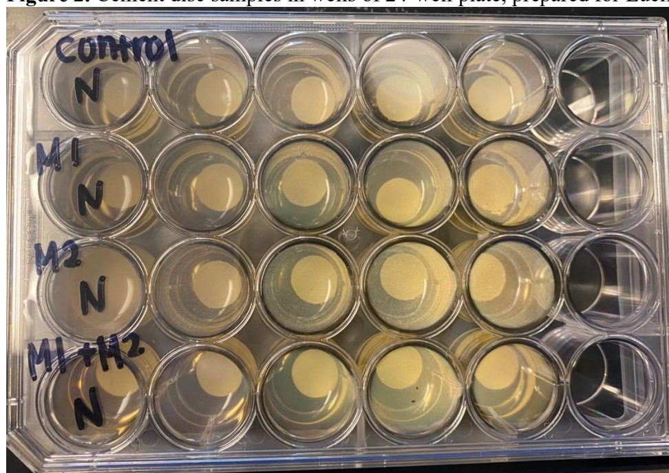
Figure 2. Cement disc samples in wells of 24-well plate, prepared for Luciferase Assay
