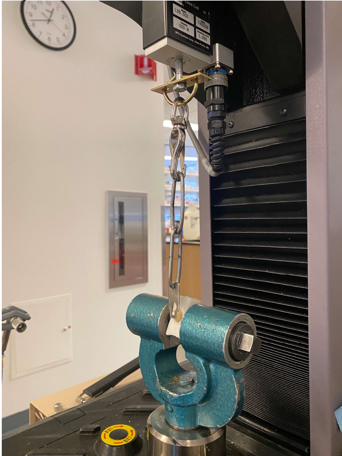
Figure 7. Mounted human premolar with bonded bracket for shear bond testing in universal testing machine.
