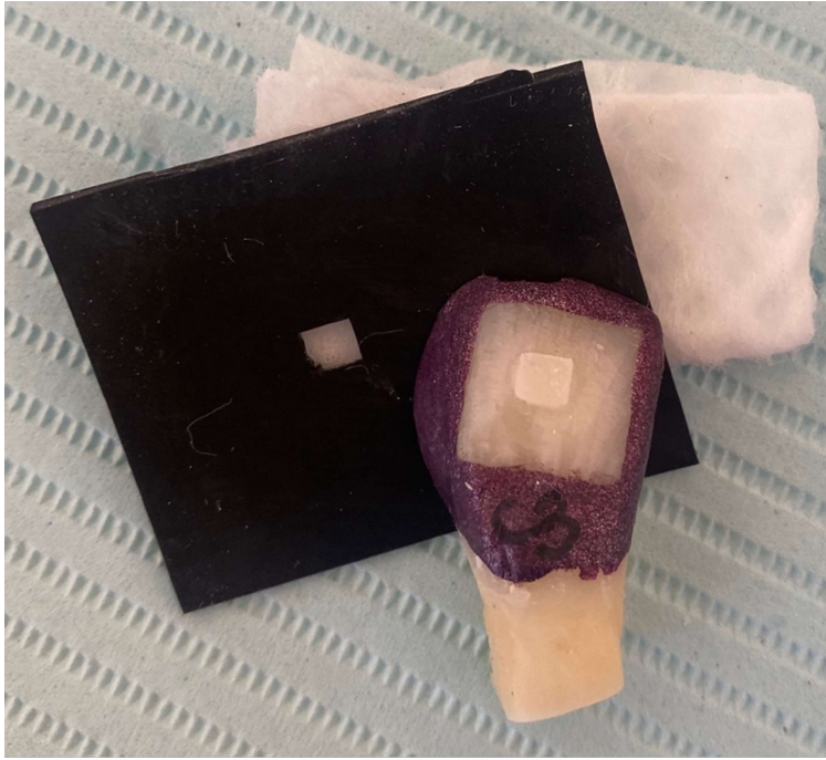
Figure 4. Black rubber template with window used to produce 3 mm x 3 mm button of cement on the bovine incisor tooth
