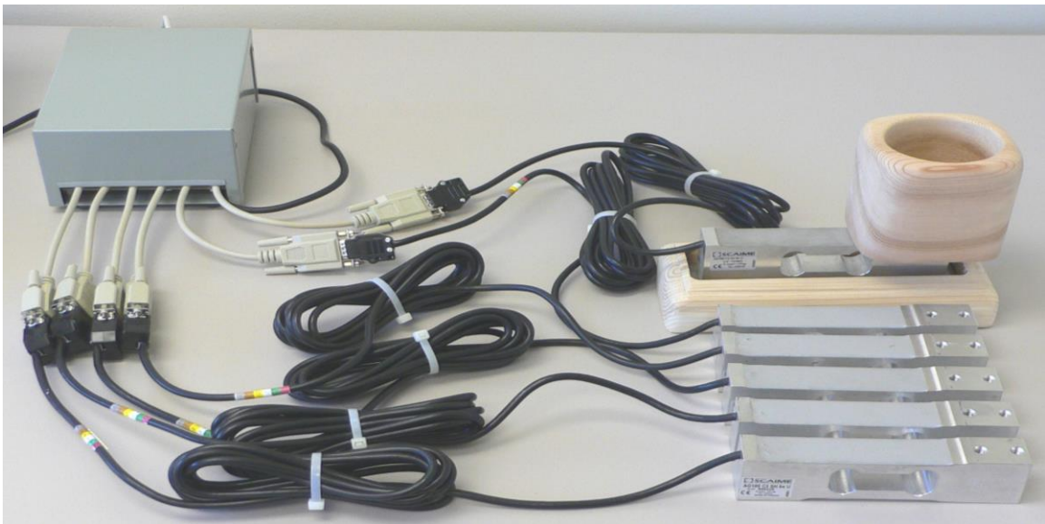
Figure 2-3. Resistive load cell design (V1). Six single point load cells shown on the right are connected to a signal conditioning box shown in the upper left via serial connectors. The upper most load cell is attached to the cedar bed attachments. The cedar block attached to the top of the upper most load cell is designed to support and contain the foot of the bed support. The base of the load cell rests in another cedar block. Not shown in the image are the 1.27cm thick steel plates bolted to the bottom of the load cells or the bolt and washer system used to securely clamp the load cells into the bottom cedar support.
