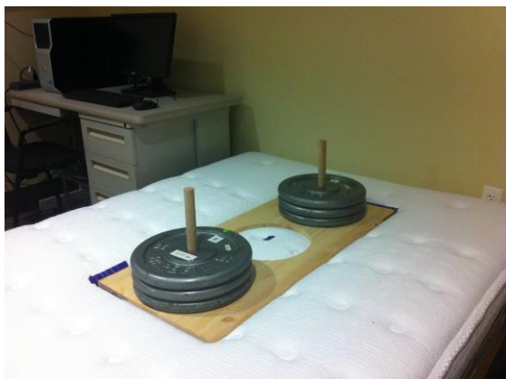
Figure 4-2. Illustration of the setup used to characterize the effect of an impulse being applied to the bed/mattress system. The wooden platform is placed on the mattress in the approximate location of an individual lying in the middle of the bed. The platform has two locations for mass to be incrementally loaded onto the bed. The center of the platform has also been removed for the application of the impulse.
