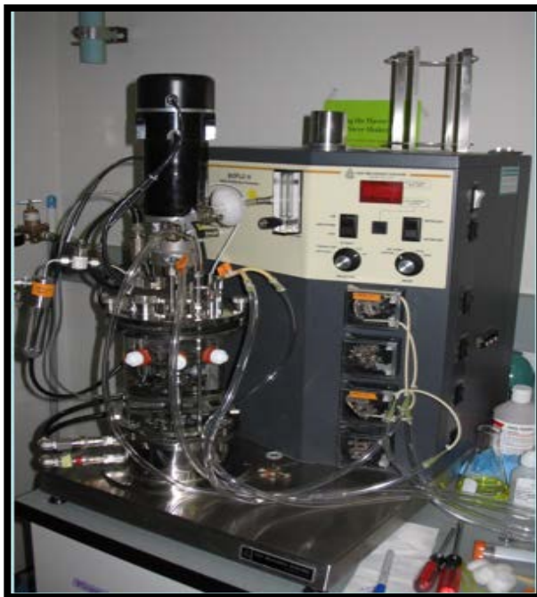
Figure 2.2 A photo showing the semi-recyclostat used to enrich Thaumarchaeota .
