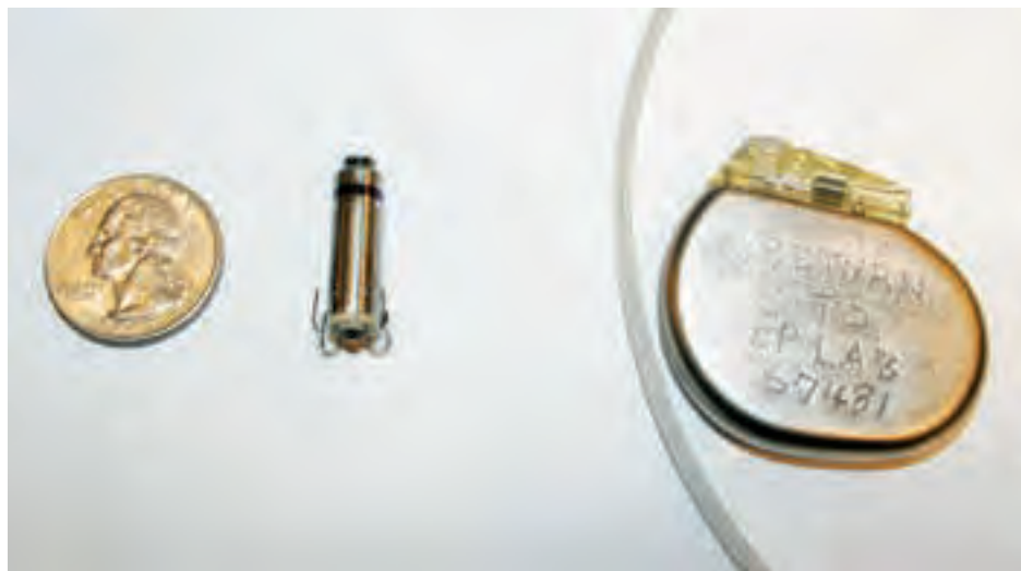
Providence St. Vincent became the Northwest's first medical center to take part in a clinical trial investigating the Medtronic Micra Transcatheter Pacing System, or Micra, which is one-tenth the size of traditional pacemakers—about the size of a large vitamin. It does not require the use of wires to connect to the heart or a surgical incision in the chest.
